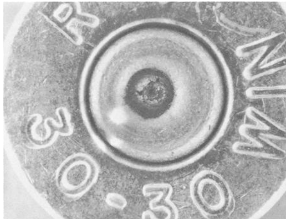
FIG. 2—Firing pin impression from fired cartridge case in rifle at crime scene.
